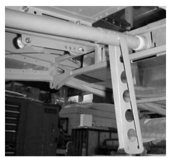
Stick assembly as viewed from under the front seat looking forward from the right side. Let the aileron driver swing freely until the wings and aileron push/pull tubes are installed.
