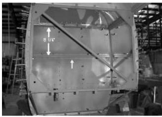
Looking back from the engine compartment at center bulkhead #3. Arrow shows the location of the center bulkhead stiffener below the hat section. Dimension shows 8½" from the bottom of the fuselage tube to the top of the hat section stiffener.
