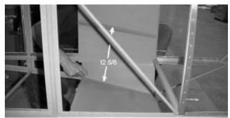
The top surface of the rudder pedal track is 12 5/8" from the forward cockpit floor and parallel to it.
