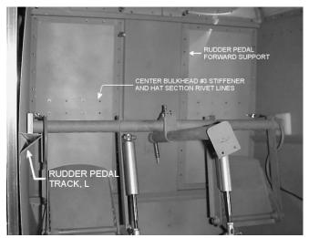
Center bulkhead #3 and rudder pedal assembly.
