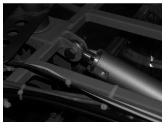
Looking forward and down from the left side of the fuselage. Shows elevator bellcrank (dark green) and tailwheel hydraulic cylinder.
