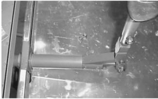
Front stick mount. Looking down from the right side. SD42BS rivets will be used to secure the forward control stick mount to the control stick torque tube.
