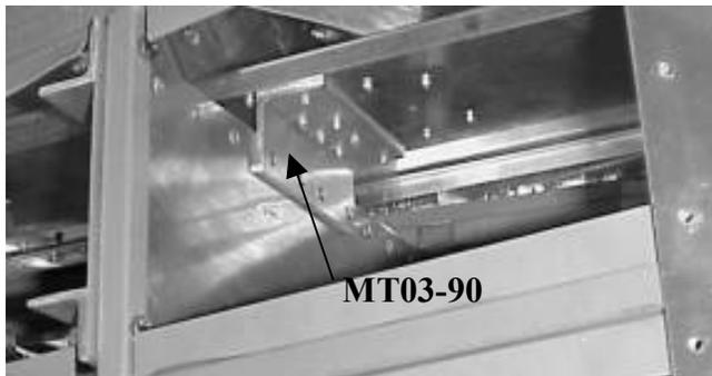
Looking back from the lower right side of the fuselage. Shows vertical stab base rib bracket. The bracket will be riveted and bonded to the center of the horizontal main spar carrythru. In this photo the vertical stab base rib is already installed.
