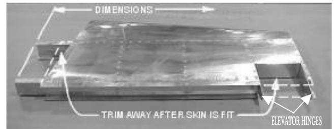
Horizontal stabilizer. The skins in the kit are rectangular and will need to be trimmed. Elevator hinges are shown in the photo. They will be installed later when the elevators are fit.
