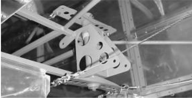
Installed rudder bellcrank. Looking back from the lower right side of the fuselage. (The cable tension has not been set in this photo.)
