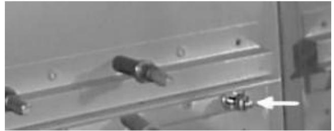
Hat section stiffener and center bulkhead stiffener nest together as shown. Note arrow showing the rudder cable anchor eyebolt from the front.
