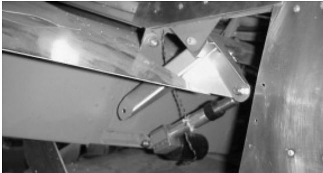
Left side flap driver and flap motor installed.
