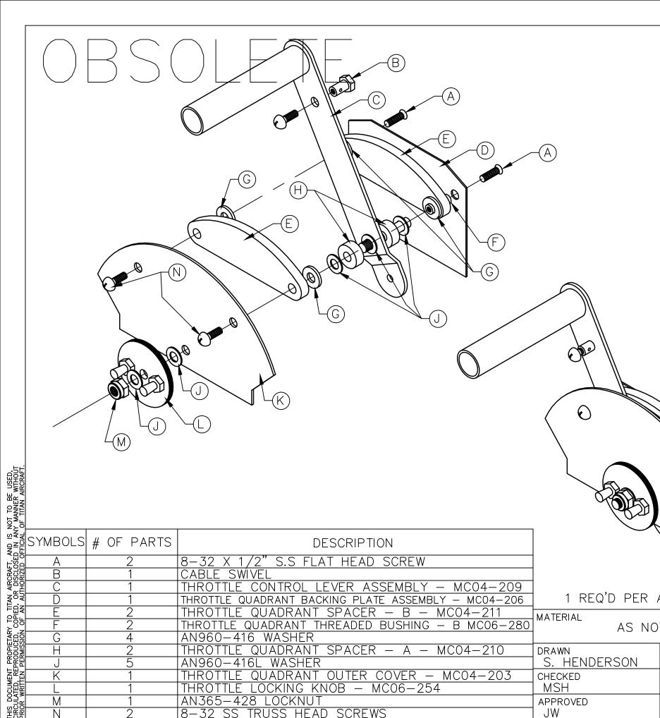
THROTTLE QUADRANT BACKING PLATE ASSEMBLY - MC04-206
